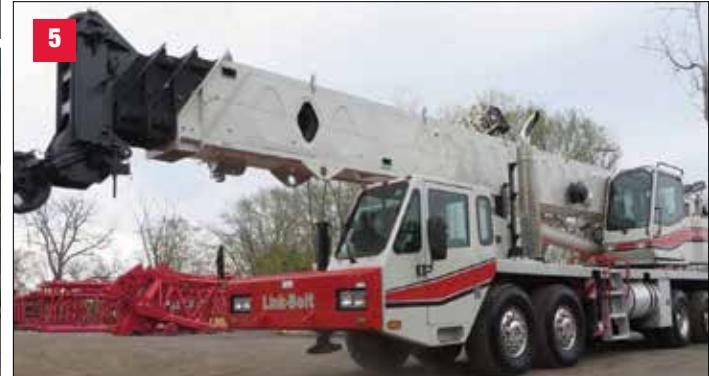
**1** **Grove TMS540E2**, S/N 224505, 2005, 40 USt, Cummins ISC 330HP, Eaton Fuller Trans, 95' Main Boom, 45' Jib, A/C & Heat. Unit #9169. Located in Orlando, FL. **\$230,000**
