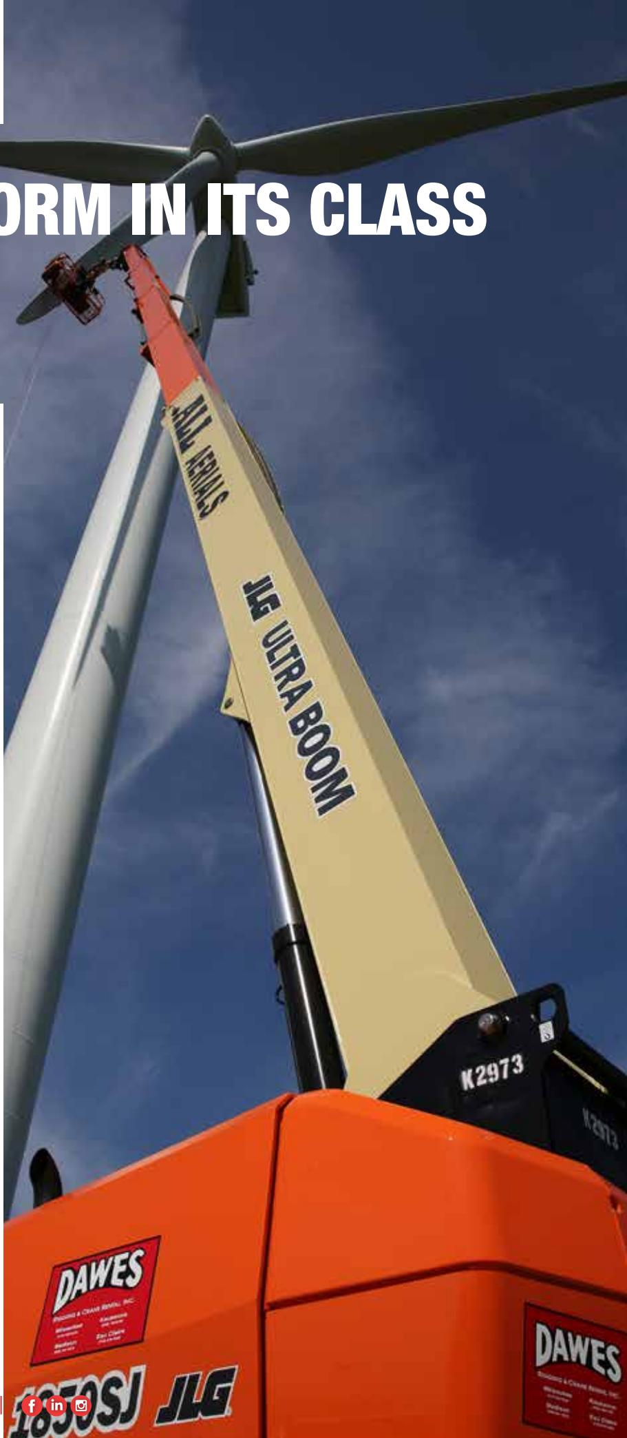
go 'up and over' something, but it may not be practical for some applications," said Kasperek. "Boom reach refers to the entire working envelope of a unit, which means the total area in which the machine's boom can operate — in this case from 10 feet to over 185 feet high." That's 82,118 cubic meters, and, according to Jerome, "an enormous working envelope."
